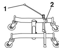
**Please note!** The brakes should always be on when you sit down or raise yourself from your chair. The brakes should be checked regularly. The rubber brake blocks can be replaced after wear and tear. Braking function may be impaired on an uneven surface.
